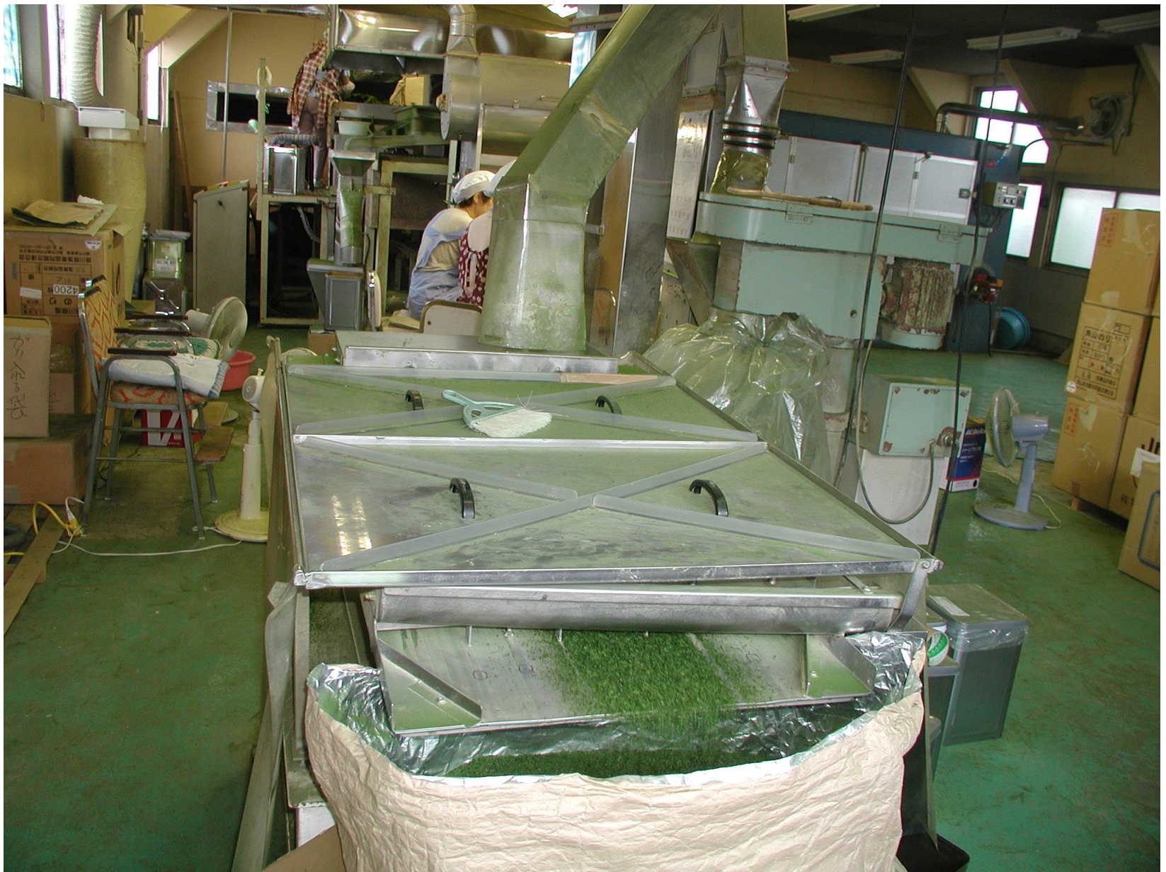
Crushed machine for Enteromorpha powder
